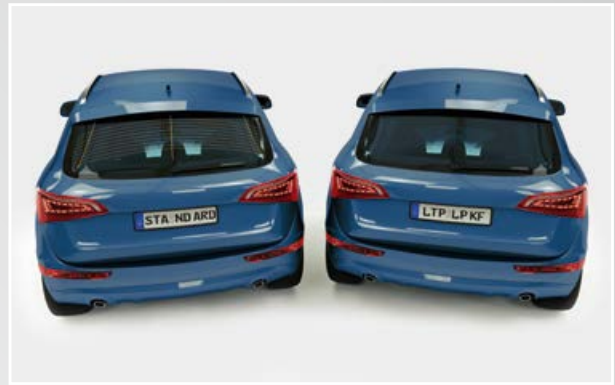
Left: conventional printing of windshield defroster; right: printing with preprinted black base
